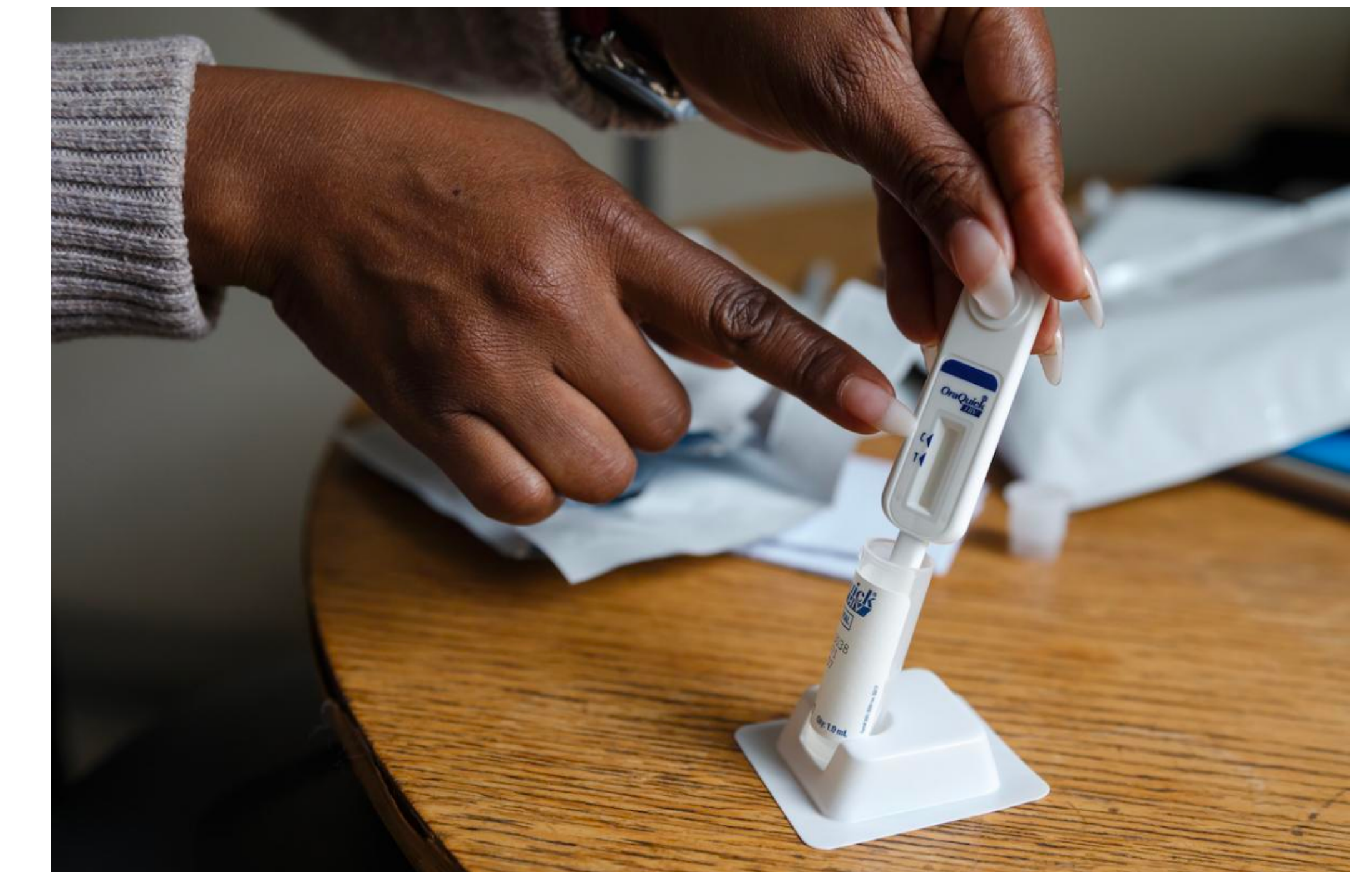
Figure 3: The OraQuick HIV Self Test helps one perform an HIV test by themselves and interpret the results in private. The test takes 20 minutes and comes with clear instructions.
