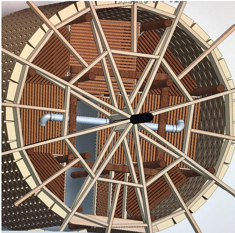
Figure 7: Looking Down into the Building at the Outlet Air Manifold
